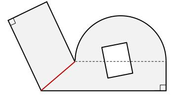
The semicircle's area  $= \pi \times 40^2 \div 2 = 2513 \text{ m}^2$ The bottom trapezium  $= \frac{1}{2} (80 + 110) \times 28 = 2660 \text{ m}^2$ The left trapezium  $= \frac{1}{2} (70 + 60) \times 40 = 2600 \text{ m}^2$ The rectangle in the middle  $= 22 \times 26 = 572$
