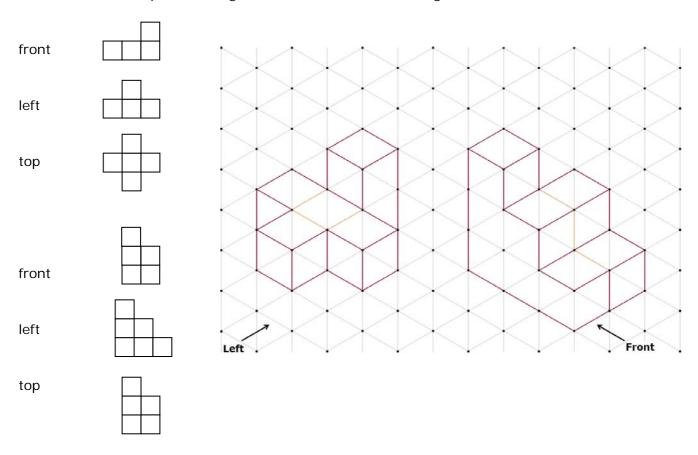
2. Convert the isometric drawings into plans
