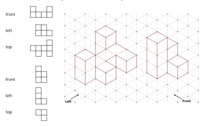
2. Convert the isometric drawings into plans
